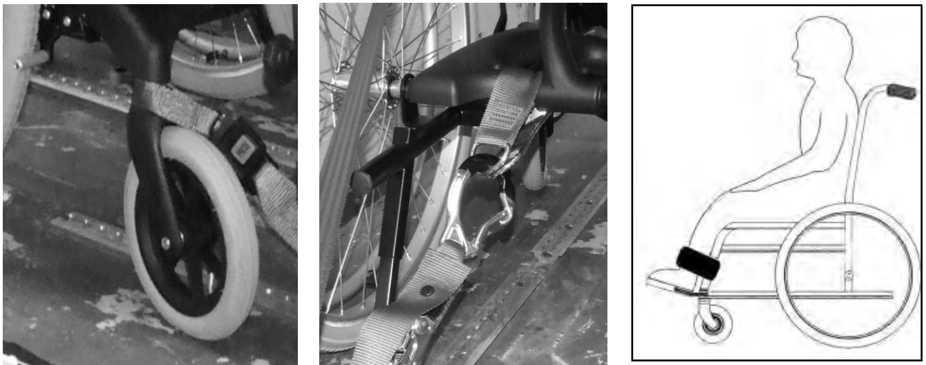
Fig 9. Pictures and graphic of Optimo indicate tie down locations front and rear of wheelchair, also the requirement for leg / calf restraints or toe straps to restrict sudden leg movement.
