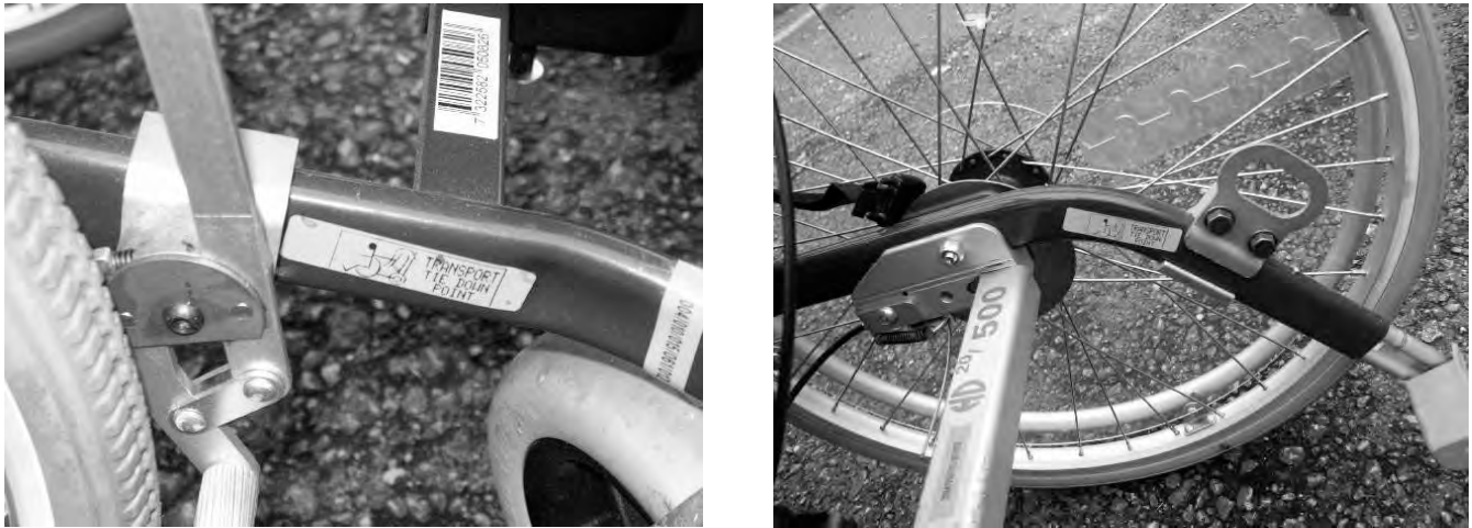
Fig 8. Pictures of Tilt in Space tie down locations, front and rear of wheelchair
