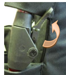
Fig 8 – Apply pressure to release and engage push handle as per above. Ensure that push handle locks are fully engaged before using the chair.
