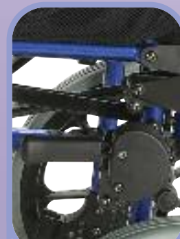
Adjustable Brake Lever Length Makes it easier to apply & release the brake
